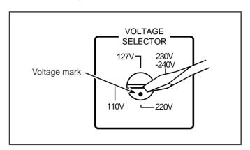
Use a screwdriver to rotate the voltage selector so the voltage number the voltage mark is pointing at is the same as the voltage where you are plugging in the unit. (See the back cover page.)
